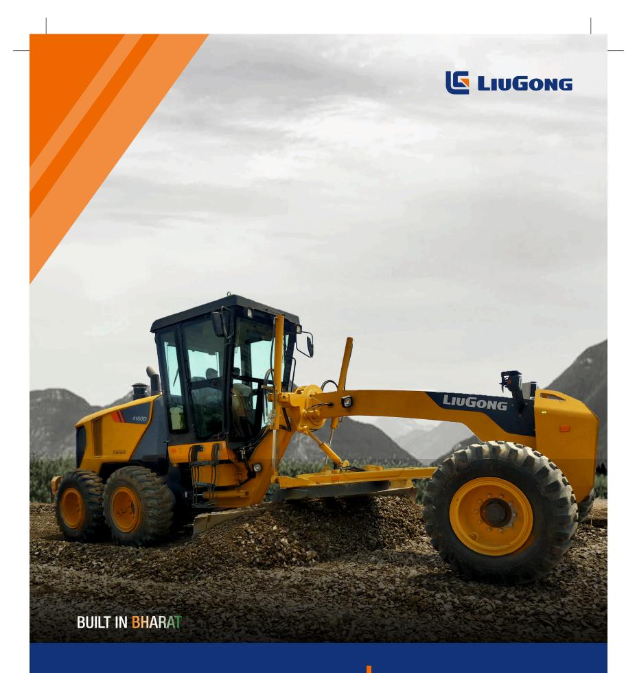
Engine Gross Power Operating Weight Standard Blade Cabin Ashok Leyland 180 hp 2200 rpm 15,000 kg 3,660 mm Air Conditioned
